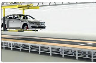
conveyor setup with height adjustable platform
