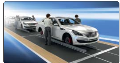
The Skid Transfer System
